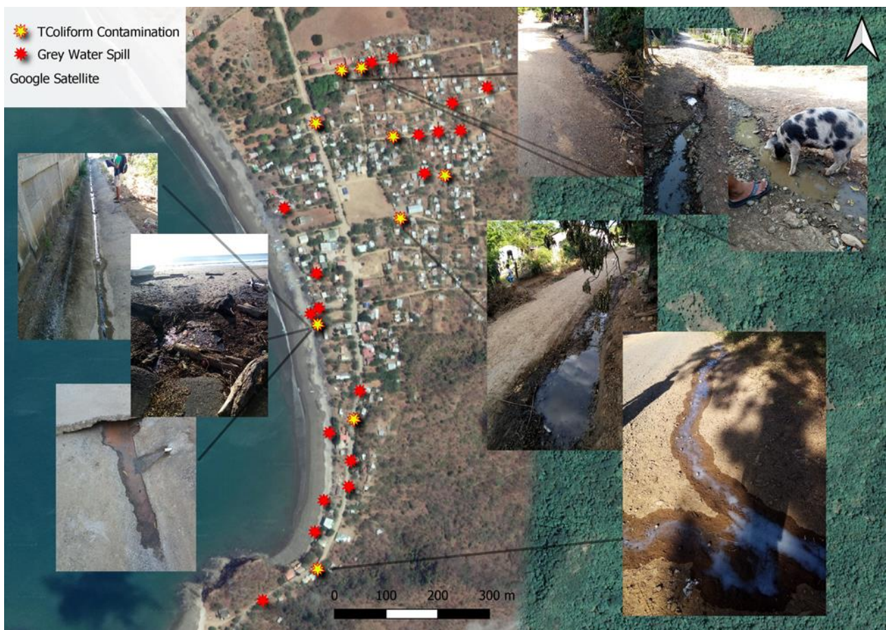
Figure 18. Grey water spill locations are labelled in red and in yellow the tested samples that revealed to be contaminated by Total Coliform.
