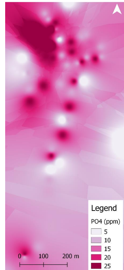
Figure 11 Phosphate Inverse Distance Weighted interpolation (IDW). Spatial analysis of the Wells measurement points.
